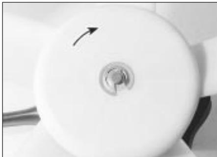
13.2 Fan blade securing clip and direction of rotation arrow
