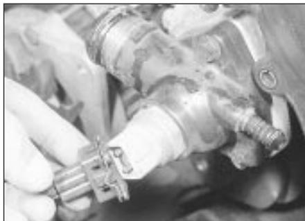
7.21 Disconnect the cooling fan switch wiring plug
