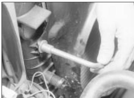
5.9 Unscrew the fan shroud/radiator retaining nuts
