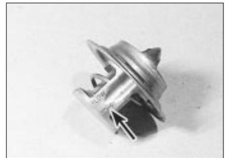
7.9 Thermostat flow direction markings (arrowed)
