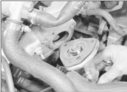
7.13 Removing the thermostat housing and gasket
