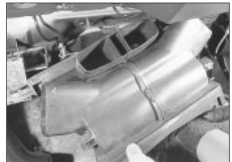
18.9 Withdrawing the heater
