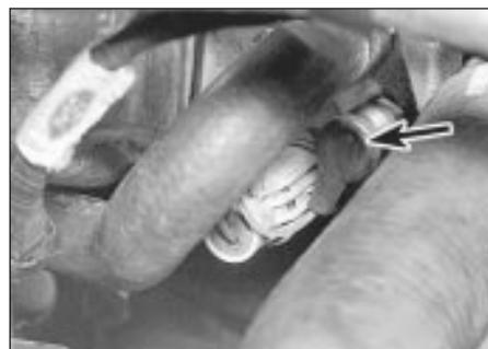
16.1 Temperature gauge sender location (arrowed)
