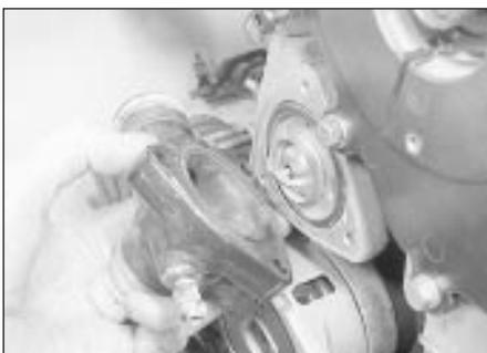
7.22 Withdrawing the thermostat housing
