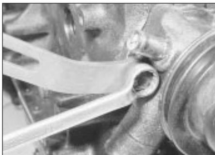
9.8 Location of the alternator adjusting link under the right-hand retaining bolt
